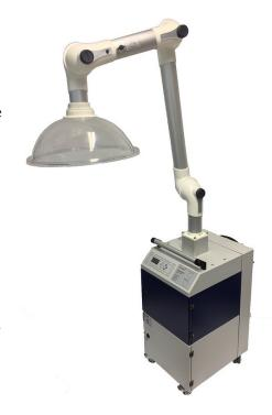
The control of the device is equipped with a digital full-text control panel with speed control, filter monitoring and operating hours counter. The swivel arm has a pipe diameter of 7.5 cm and a reach of 85 cm. The round, transparent dome hood has a patient-friendly and even recommended diameter of 50 cm.
